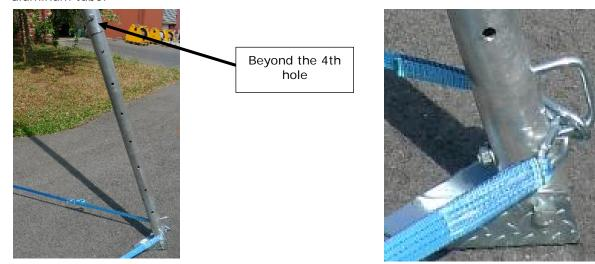
Last, hang the hoist at the point of anchoring of the head
